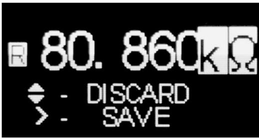
Figure 2-33: Save Reference Resistance Value from Inputting
