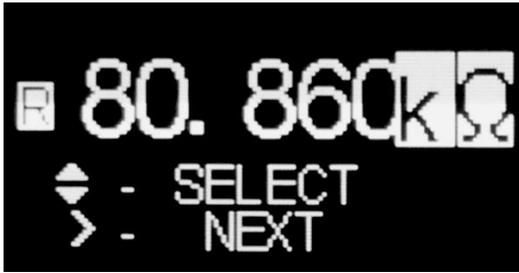
Figure 2-32: Input Unit for Reference Resistance Value
