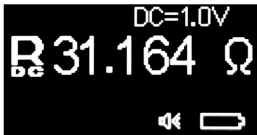
Figure 3-12: Display of DCR Measurement
