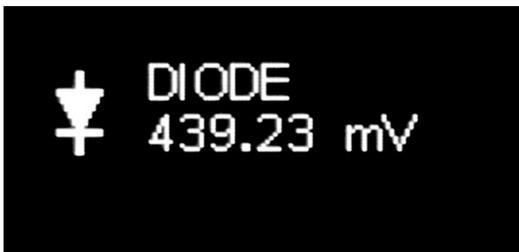
Figure 3-13: Display of Diode Measurement (Good Diode)
